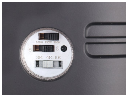
Power, CCT, and Photocell Selector Switches
